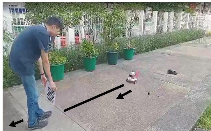
Figure 30. Setup of Follow-Me test (Moving Marker)
