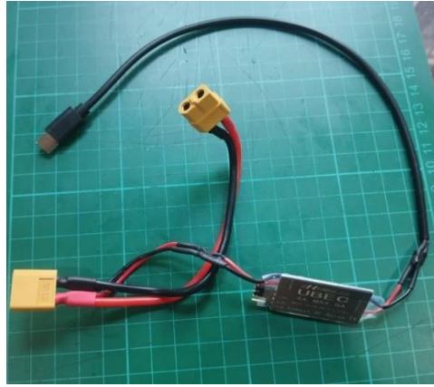
Figure 11. Power cable for the mainboard and RPi
