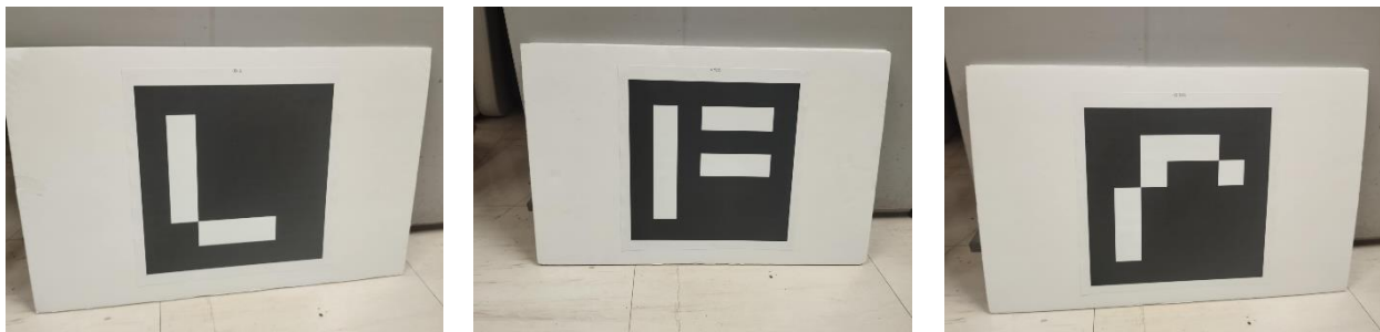
Figure 17. Multiple Markers (a) Left Marker - ID #3 (left), (b) Forward Marker - ID #272 (middle), (c) Right Marker - ID #836 (right)
