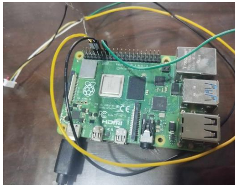
Figure 12. 6-pin JST connected to jumper wire for Pixhawk-RPi connection
